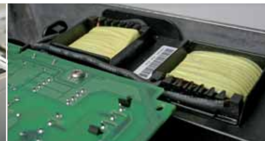
Built-in circuit chokes reduce the impact on the supply network and increase the lifetime of the drive.
