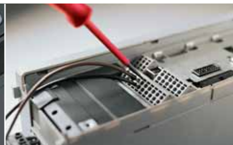
Spring-loaded connectors save considerable time and costs, both in installation and service.
